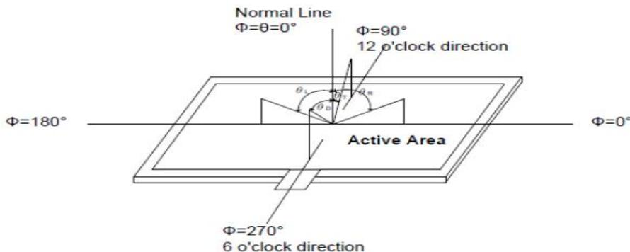
Viewing angle is the angle at which the contrast ratio is greater than 10. The angles are determined for the horizontal or x axis and the vertical or y axis with respect to the z axis which is normal to the LCD surface
