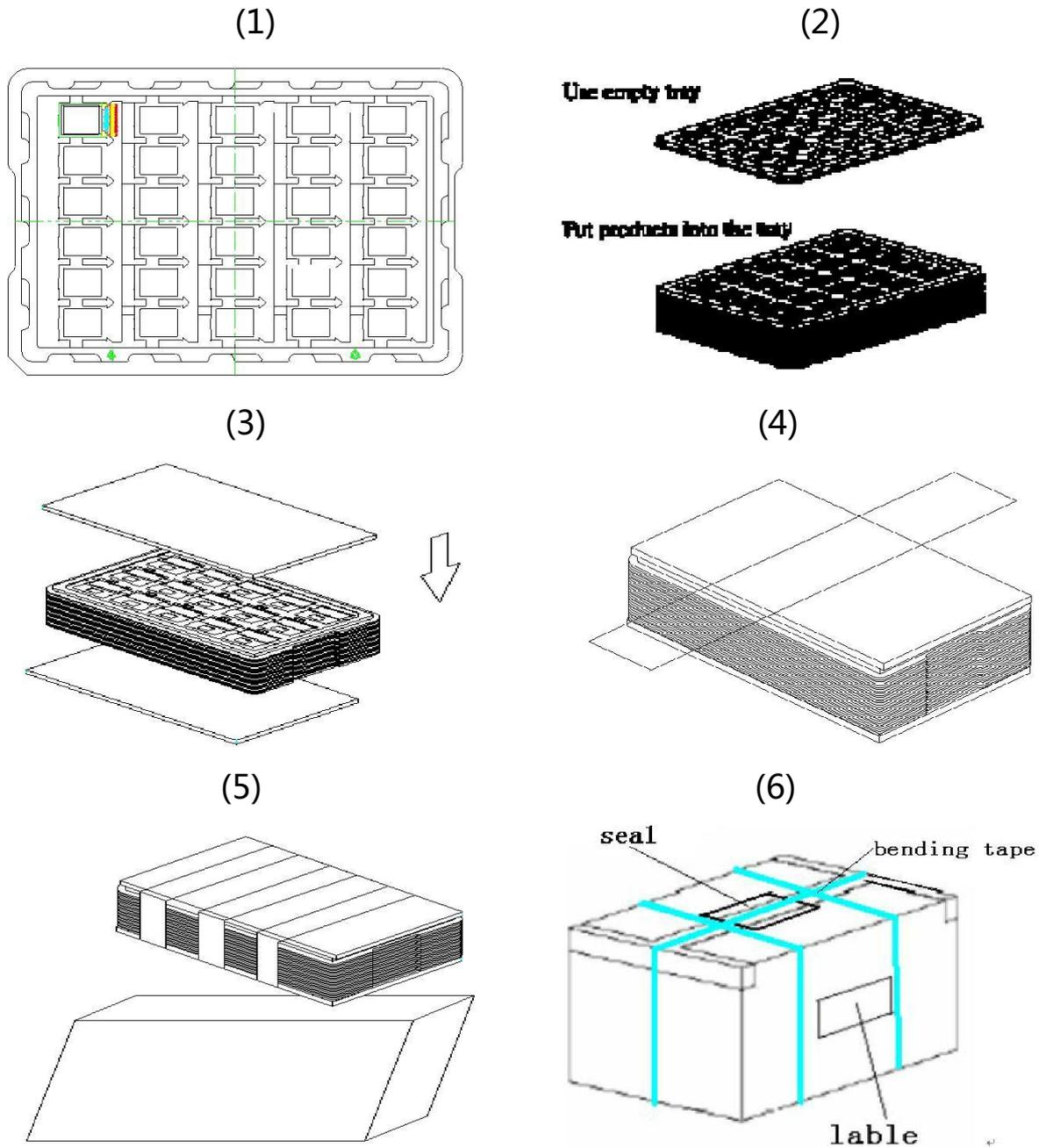
1. Put module into tray cavity.
