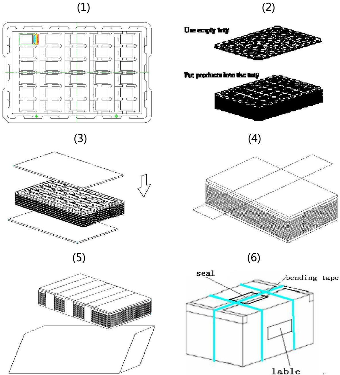
1. Put module into tray cavity.
